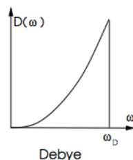
Figure 1: Density of states (DOS) of phonon in a solid
